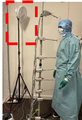
Solution 4: Mixing wall fan
