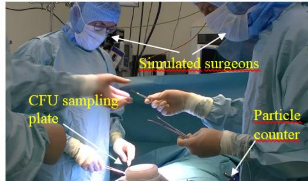
Figure 2 The locations of the measurement instruments for CFU measurement and particle measurement
